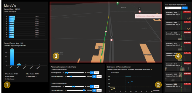
Figure 9: The primitive version of MaraVis consists of (1) a marathon overview, (2) an anomaly detection view, (3) a camera shot view and (4) a list of anomalous runners.
