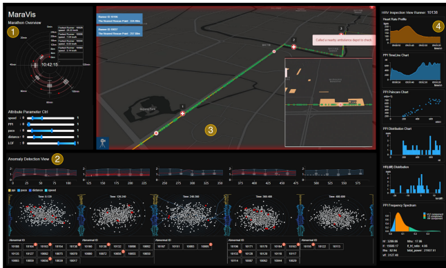
Figure 5: The full MaraVis system contains four coordinated views: (1) a marathon overview, (2) an anomaly detection view, (3) a camera shot view, and (4) an HRV inspection view.
